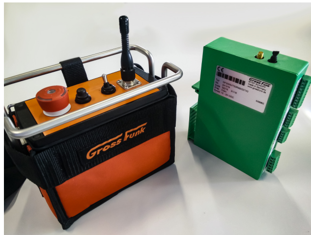
Figure 6: RES sender & receiver
